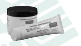
**120-\*) Thermal Compound** – The 120- Thermal Conducting Compound is a zinc oxide-filled, dielectric, silicone oil-based compound that facilitates heat transfer by filling voids and gaps between mating surfaces. The operating temperature range is -40° to 200°C (-40° to 392°F). It is available in a 5 oz tube or 2 & 8 oz jars.
